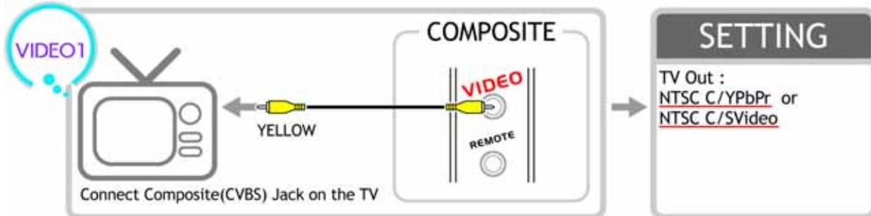
Using Composite Video(CVBS, Yellow) : An easy way of transferring video signals.
